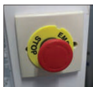
Emergency stop button
