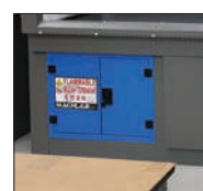
Flammable/corrosive chemical safety cabinet
