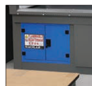
Corrosive chemical safety cabinet
