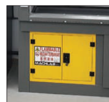
Flammable/corrosive chemical safety cabinet
